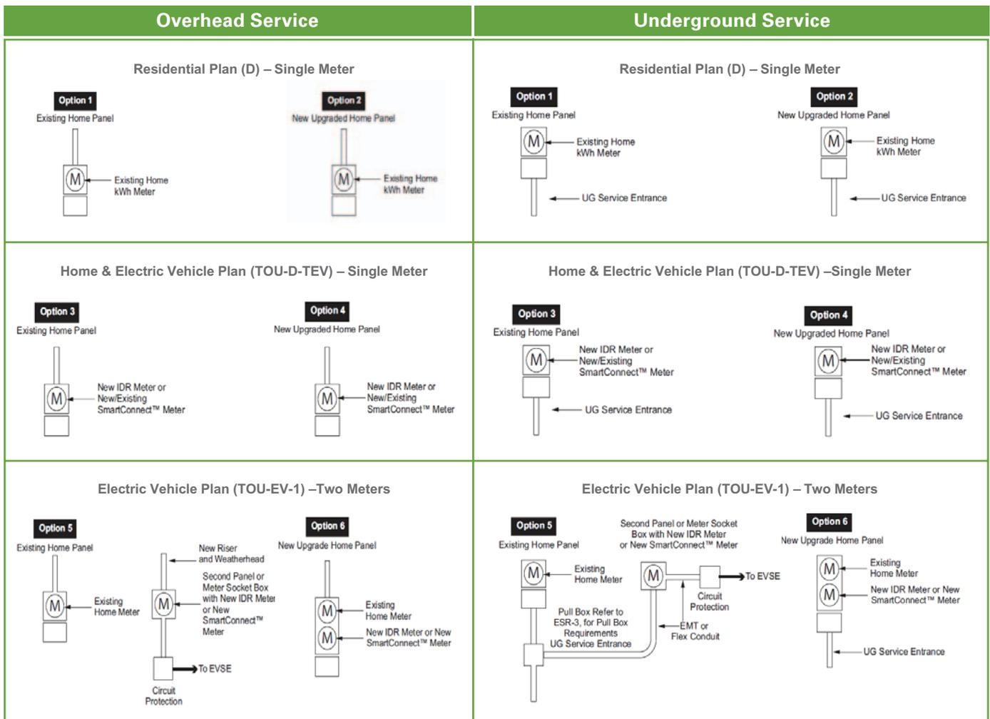
**Note 1:** SCE provides *only a single service line* for all panel configurations, regardless of whether one or two panels are installed.
