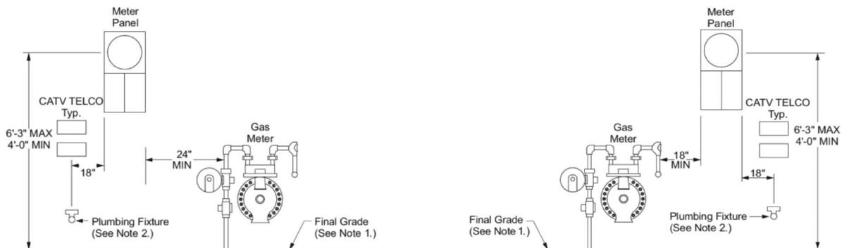
**Figure 5–5: Surface-Mounted or Semi-Flush Meter Installation**
