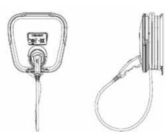
16.5" x 16.5" x 6.5" (front of unit excluding connector) 15" minimum clearance recommended for connector when inserted
